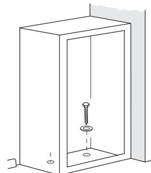
5. Secure the safe with fasteners and replace carpeting.
