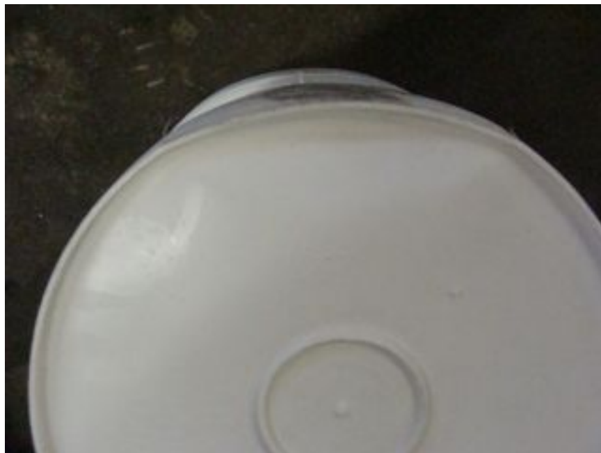
Photo No. 6 – Slight Distortion On the Drum After the Side Face Drop
