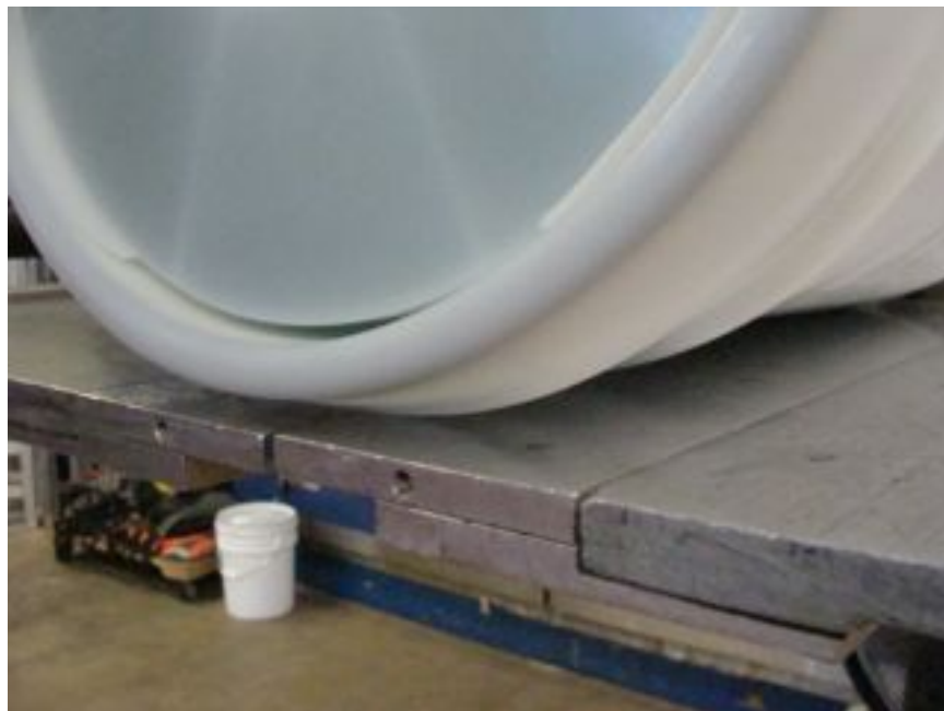
Photo No. 4 - Closure Position During the Flat Side Drop Test
