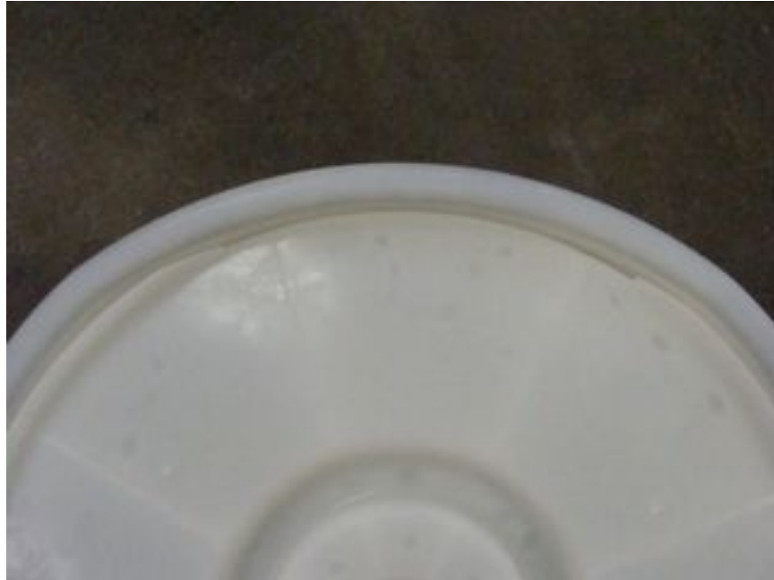
Photo No. 5 – Slight Distortion on Lid After the Diagonal Drop
