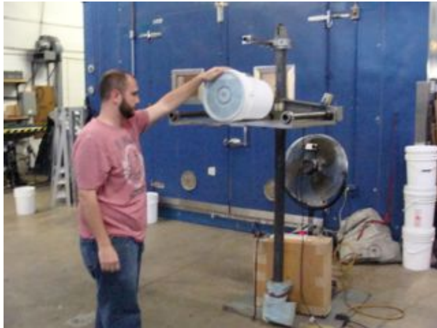
Photo No. 3 - Flat Side Drop Setup
