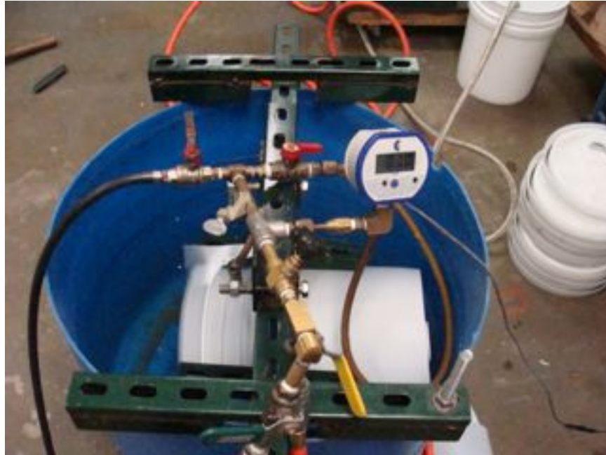
Photo No. 7 - Leakproofness Test Setup
