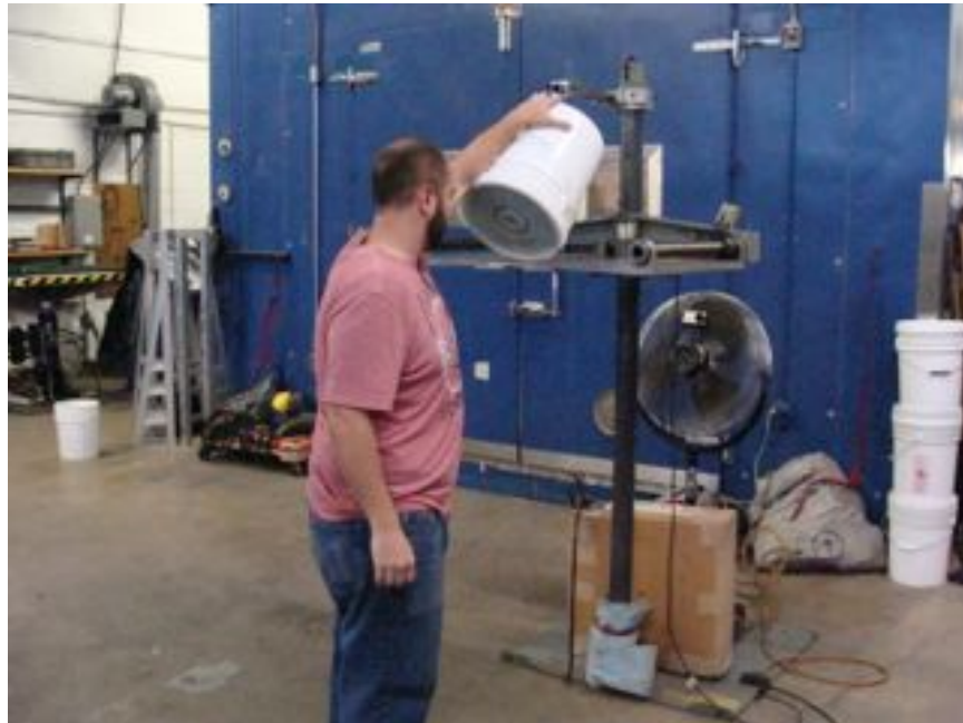
Photo No. 1 - Top Diagonal Drop Setup
